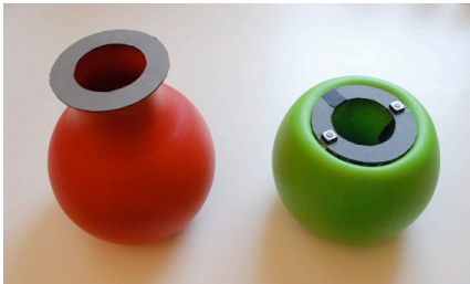
figure 2: Balloons, in a droplet (L) and bubble (R) shape have a pushbutton ring at their opening to detect a user's face against the balloon. It houses the force sensor, camera, and an LED.
