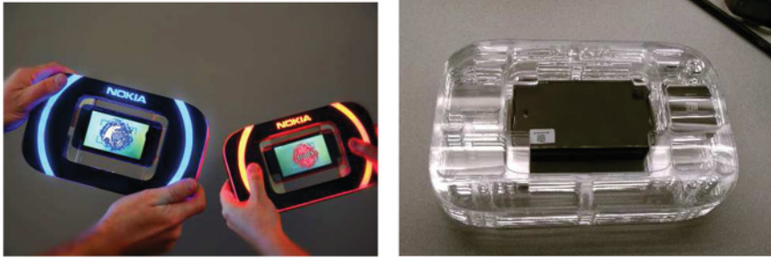
Fig. 10. Form factor of the communicator. (Left) Each communicator glows to represent the role of the player, either Agent Red or Agent Blue. (Right) A clear version of the housing makes the Ariane sensor box visible to the right of the N900.
